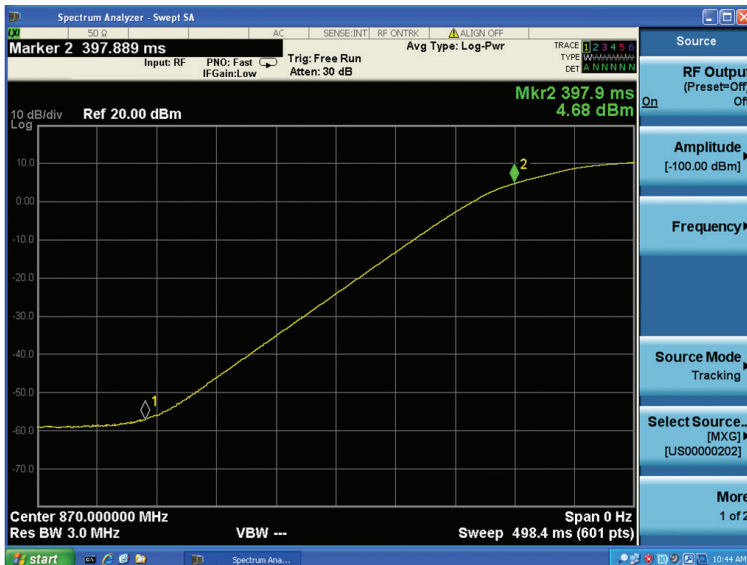
Figure 13. The power sweep at a fixed frequency tests the amplifier’s cut-off level, linear region, and gain compression
