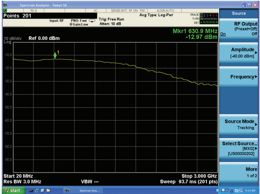
Figure 8. "Standard sweep" for measure the frequency responses of the amplifier
